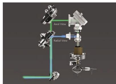
The Dual View system measures the axial view for low detection limits and the radial view for extended working ranges.
